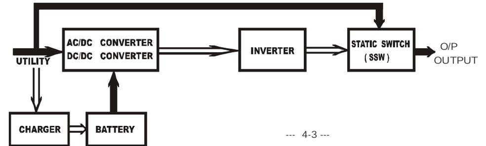
Normally, an inrush current is generated when switching on the connected device. If the UPS is in 105~120% loading, it will switch to bypass mode in 60 seconds. If The UPS is in 120%-150% loading, it will switch to bypass mode in 10 seconds. If The UPS is over 150% loading, it will switch to bypass mode immediately. The Utility LED, Bypass LED and Over Load LED light up. If overload condition is eliminated by reducing the load to 80%~90%, the UPS will switch back to Inverter mode automatically.
