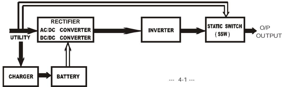
When Utility is normal, the AC source is rectified to DC, partially fed into the charger to charge battery and partially fed into inverter. The inverter reverts the DC to a cleaned and pure AC to supply energy to the load connected. The Utility LED and Inverter LED Light up.
